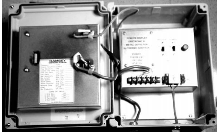
Figure B–2. Interior of the Remote Front Panel Enclosure
